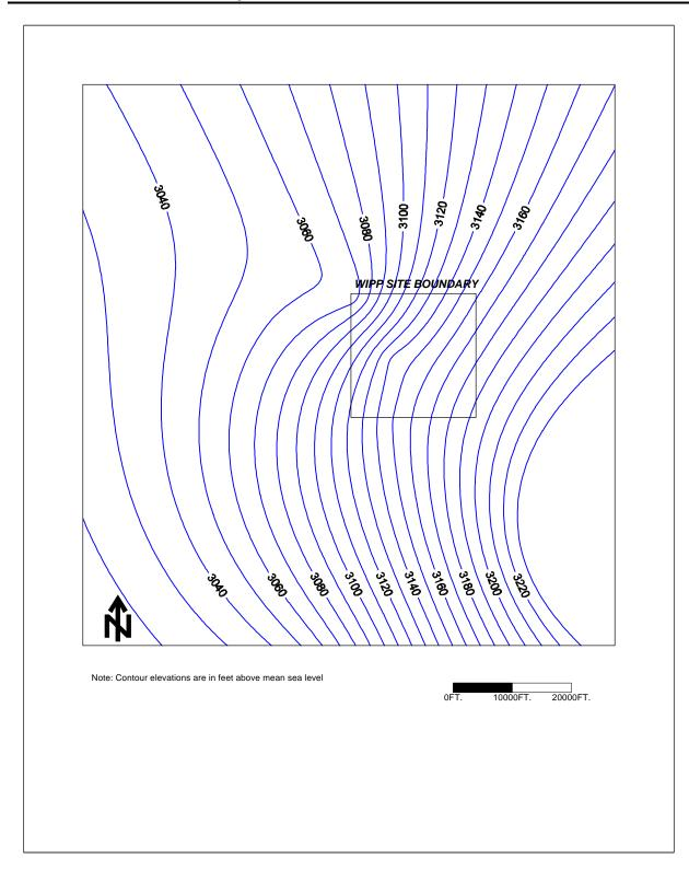
Figure 7.4 - Potentiometric Surface of the Magenta Dolomite Member of the Rustler Formation Near the WIPP Site as of December 1998 (adjusted to equivalent fresh water head)
