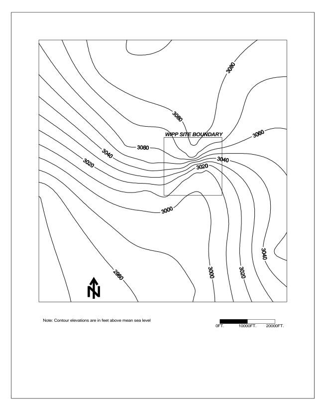
Figure 7.3 - Potentiometric Surface of the Culebra Dolomite Member of the Rustler Formation Near the WIPP Site as of December 1998 (adjusted to equivalent fresh water head)
